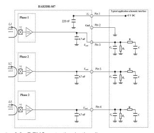
$C_{\rm L}$ < 2.2 nF EMC protection (optional) RC Low pass filter (optional)
